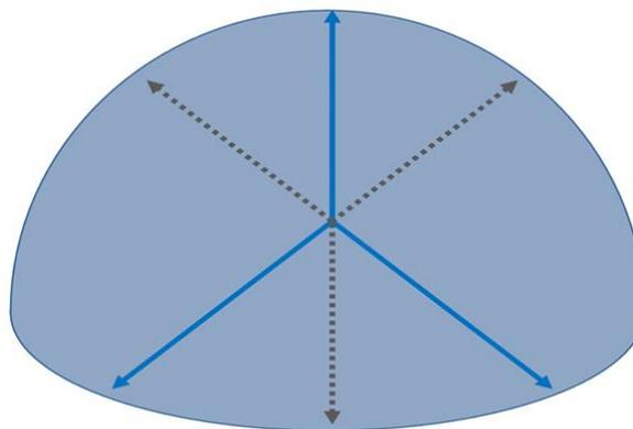
The effective diameter of a trilobed mold is easily detected by use of a three-point bore gauge.
