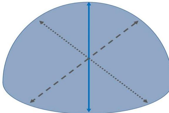
Trilobing is not easily detected when using a two-point bore gauge.
